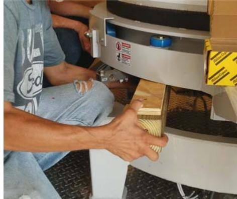
Remove the load cell pads from the top of each leg and put the pads in a box for transport. Mark the box for easy identification and be sure not to lose it. Removing the load cell pads assures that they do not come lose during transport. Ensure that each load cell is NOT making contact with any surface. If necessary, adjust the position of the base slightly so that all load cells are clear of any contact.
