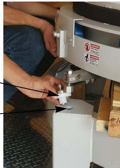
Load cell pad with ball mount
