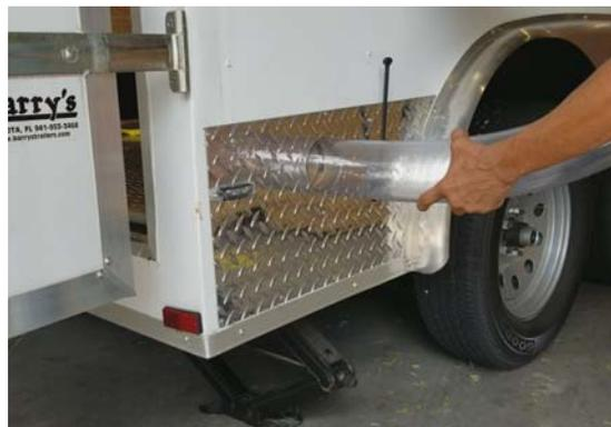
Secure the discharge tube to the coupler by tightening the coupler wing nut.
