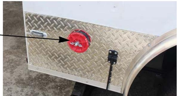
Insert a section of discharge tube through the hole and into the coupler on the inside of the trailer. Choose either a straight section or the 90° curved section, whichever best suits your specific layout requirements.
