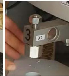
While one person lifts a side of the base, the other person must insert a load cell pad into the hole at the top of each leg on that side of the base. Repeat this for the other side of the base so that all four load cell pads are installed.
