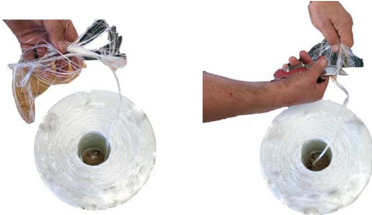
If there is loose roving coming from the outside of the bobbin, tuck it under the plastic wrap.
