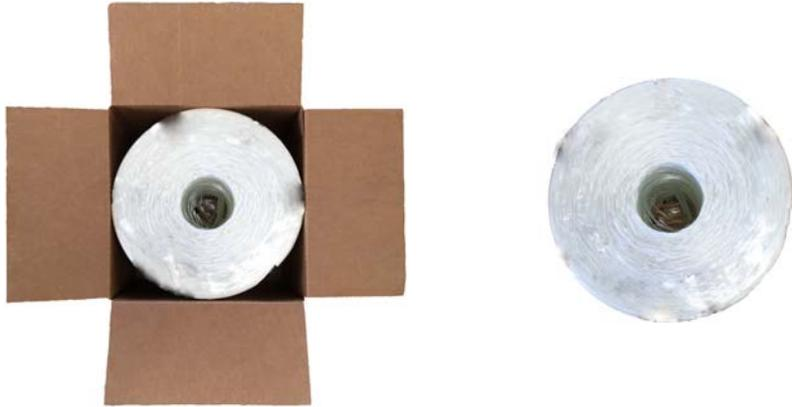
The roving will feed from the center of the bobbin. Pull the loose roving out of the center of the bobbin and trim off any excess/knotted portion of the roving.
