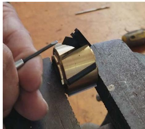
7. Insert a new blade and the spacer into the groove - the blade goes to the right side of the groove and the spacer just behind (or to the left of) the blade.
