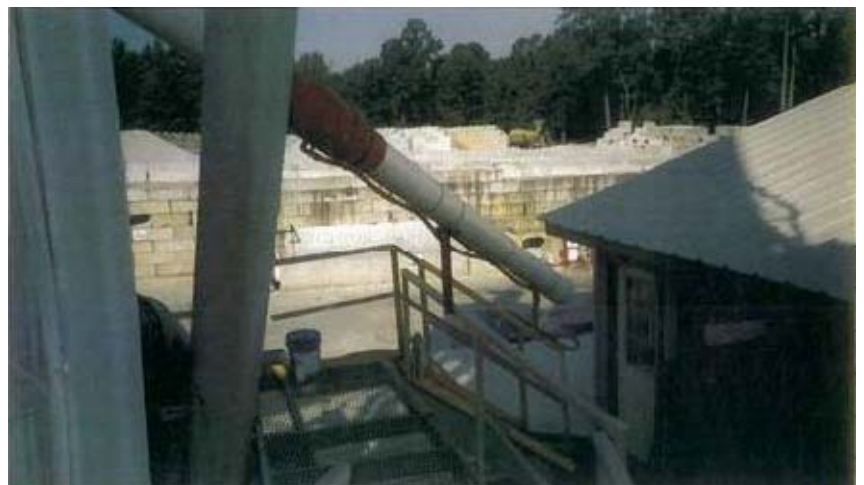
Initial pipe section should be 5 to 10 feet long to create vacuum.
